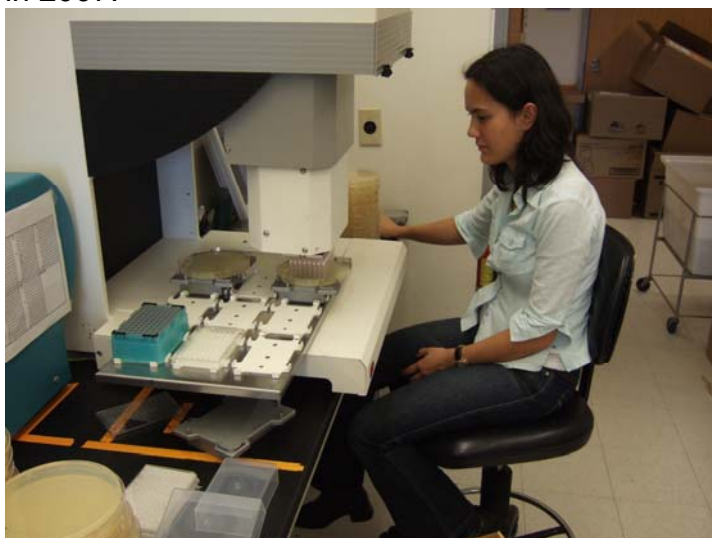
Julie-Anne using one of the Genmate robots to spot yeast strains onto an agar plate for yeast two-hybrid mating experiments.
